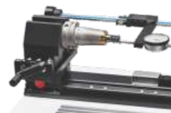
Length Adjustment Fixture with Dial Indicator
